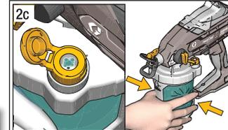
**Note:** Tilt the sprayer such that the VacuValve is the highest point so that all air in the FlexLiner can be fully evacuated.
