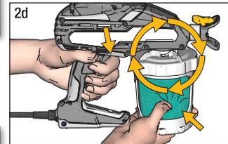
**Note:** This will purge all air from the pump and cup. Paint will not spray out, but will recirculate through the pump and back into the cup.
