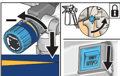
**6** Turn Pressure Control Knob to lowest setting and release trigger. Engage Trigger Lock. Turn the Prime/Spray Valve to PRIME and turn Power Switch OFF.
