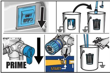
**1** Turn Power Switch OFF. Place Suction and Drain Tubes in waste pail. Turn Prime/Spray Valve to PRIME. Turn Pressure Control Knob to START position. Trigger gun into a waste pail.
