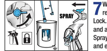
**7** When paint comes out of gun, release trigger. Engage Trigger Lock. Transfer Drain Tube to paint pail and attach to Suction Tube. Rotate Spray Tip back to **SPRAY** position and ensure Spray Tip Guard is tight.
