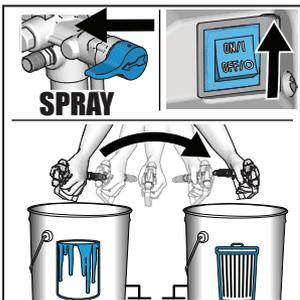
**5** To save paint in hose, disengage Trigger Lock and trigger gun into paint pail, turn Prime/Spray Valve to SPRAY and turn Power Switch ON. When water comes out of gun, keep gun triggered and aim into waste pail. Continue to flush until water runs clear.
