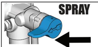
**6** Turn the Spray/Prime valve to SPRAY position for storage. Turn Power Switch OFF and unplug sprayer from outlet.
