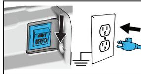
**1** Turn Power Switch OFF and plug sprayer into a grounded outlet.
