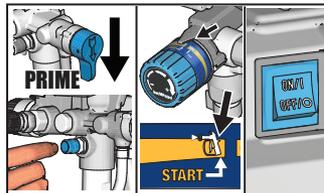
**3** Turn the Prime/Spray Valve to the PRIME position. Press the PushPrime™ button twice to loosen inlet valve ball. Turn Pressure Control Knob to START position. Turn Power Switch ON.
