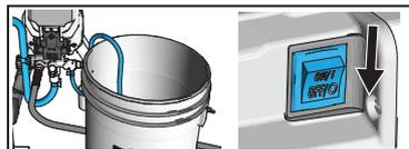
**4** Allow fluid to flow up the Suction Tube and out of Drain Tube for 30-60 seconds. Turn Power Switch OFF.
