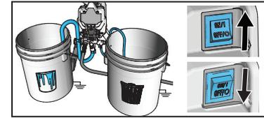
**5** Submerge Suction Tube into paint. Turn Power Switch ON and watch for paint to come out of the Drain Tube. Turn Power Switch OFF.
