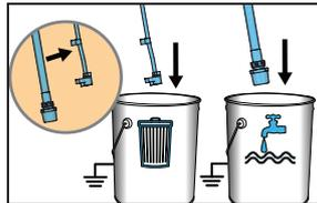
**2** Separate Drain Tube (smaller) from Suction Tube (larger). Place Drain Tube in a waste pail. Submerge Suction Tube into pail filled with water for water-based material, or mineral spirits if spraying oil-based material.
