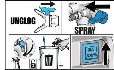
**6** Rotate Spray Tip to **UNCLOG** Position. Disengage Trigger Lock. Point gun into waste pail, pull and hold trigger. Turn the Prime/Spray Valve to **SPRAY** position and turn Power Switch ON.
