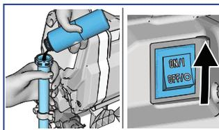
**3** While holding the Suction Tube above the sprayer, pour approximately 2 ounces (60 ml) of Pump Armor into the Suction Tube and turn Power Switch ON.
