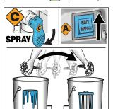
5 To save paint in hose, disengage Trigger Lock and trigger gun into paint pail, lower Prime/Spray Valve to SPRAY and turn Power Switch ON. When water comes out of gun, keep gun triggered and aim into waste pail. Continue to flush until water runs clear.
