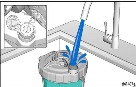
**NOTE:** Be sure to clean inside the VacuValve reservoir. If the VacuValve air hole becomes clogged, use a paper clip to clean hole.
