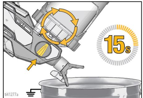
5. To spray cleaning fluid, refill cup assembly half-full of cleaning fluid and reattach to sprayer.
