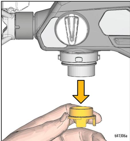
3. Reinstall the Pump Filter into the pump. Set sprayer on a rag.
