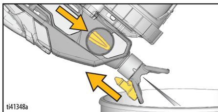
9. Turn Prime Valve to PRIME position to relieve system pressure and immediately back to SPRAY position for storage. Unplug Power Cord.
