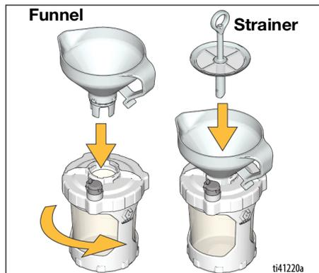
4. The Strainer's Air Tube will prevent paint from overflowing the cup. Fill the cup as follows:
