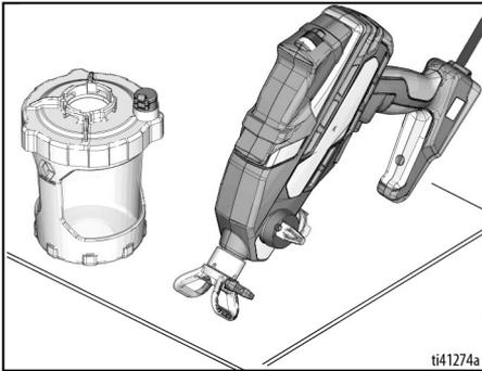
3. Remove Cup Lid and pour extra paint back into paint can. Clean all parts with warm water.
