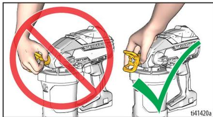
Adjust the Spray Tip Guard for the desired vertical or horizontal spraying direction.
