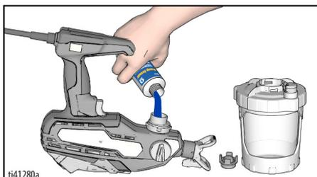
6. Install clean Pump Filter into pump.
