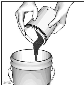
5. It is recommended to dispose of the used FlexLiner (4) and install a new one. If reusing, clean by wiping all excess fluid from FlexLiner (4).
