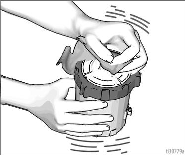
11. Wipe clean and dry all components of FlexLiner System. Properly dispose of cleaning fluid.
