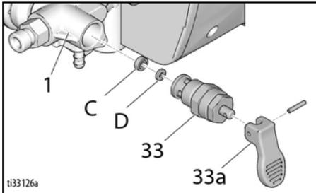
6. Apply sealant to threads of new valve stem assembly (33). Install valve assembly in pump housing. Torque to 220-250 in-lb (24.9-28.2 N•m).
