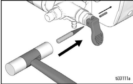
4. Remove Prime/Spray Valve handle (33a).
