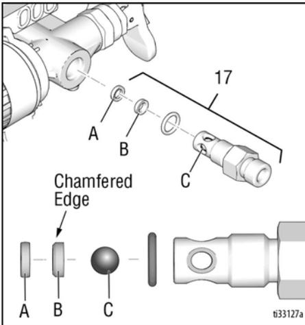
5. Thread new outlet valve (17) into pump housing (1). Torque to 290-310 in-lb (32.8-35.0 N•m).
