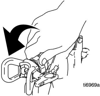
3. Use the SwitchTip (D) to remove OneSeal (SL) from the tip guard (A).
