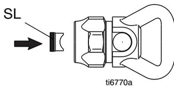
4. Use the end of SwitchTip (D) to press OneSeal (SL) into tip guard (A) with the curve matching the tip bore (TB).
