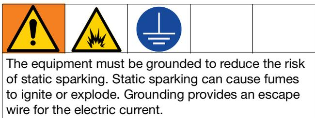
**Spray Gun:** ground through connection to a properly grounded fluid hose and pump.
