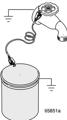
**Maintain Grounding Continuity:** When flushing or relieving pressure, hold a metal part of the gun firmly against the side of a grounded metal pail, then trigger the gun.
