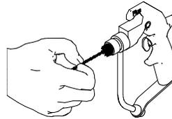
9. Grease the o-rings of the new needling using a non-silicon grease.
