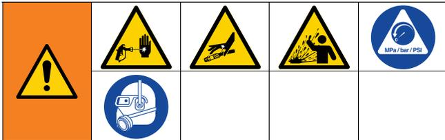
This equipment stays pressurized until pressure is manually relieved. To help prevent serious injury from pressurized fluid, such as skin injection, or splashing fluid, follow the Pressure Relief Procedure when you stop spraying and before cleaning, checking, or servicing the equipment.
