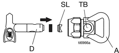
5. Insert SwitchTip (D) into tip bore. Firmly thread the assembly onto the gun, then hand tighten.
