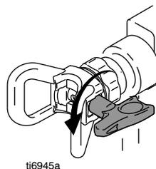
7. Disengage the trigger lock. Trigger the gun into a pail to verify the tip is clear.
