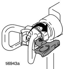
3. Disengage the trigger lock.
