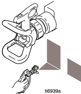
2. Before spraying, verify tip guard is tight. Tighten if necessary.
