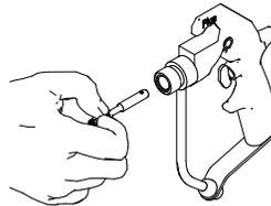
**NOTE:** An insertion tool is provided in your needle kit. This tool helps prevent damage to the needle.
