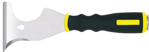
BG1 (09081) EXTENDABLE HEAVY-DUTY 8-IN-1 TOOL, HAMMER END Serves as a spreader, chisel scraper, crack & can opener, roller cleaner, nail puller; removable hammer end reveals a threaded socket for use with extension pole.
