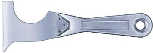
TG1 (08008) 5-IN-1 TWO-PIECE STAINLESS-STEEL PAINTER'S MULTI-TOOL Serves as a scraper, chisel, crack & can opener, roller cleaner & spackle/adhesive spreader.
