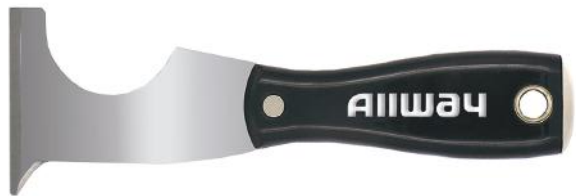
NXG1 (09507) 6-IN-1 ERGONOMIC PAINTER'S MULTI-TOOL Serves as a scraper, chisel, crack & can opener, roller cleaner & spackle/adhesive spreader; die-cast hammer end.
